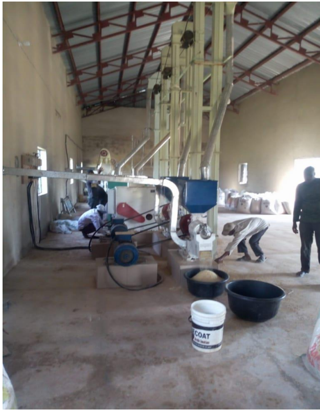
Multi stage rice milling - using semi integrated modular rice mills
