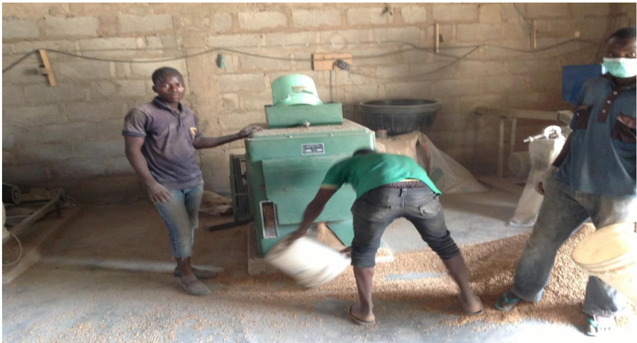
Paddy de-stoners - using medium scale (1-2 t/hr) unit electric de-stoners
