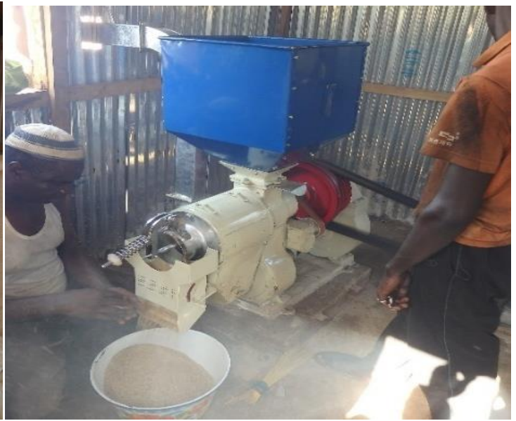
Single pass Rice milling and polishing -using engleberg and improved machines
