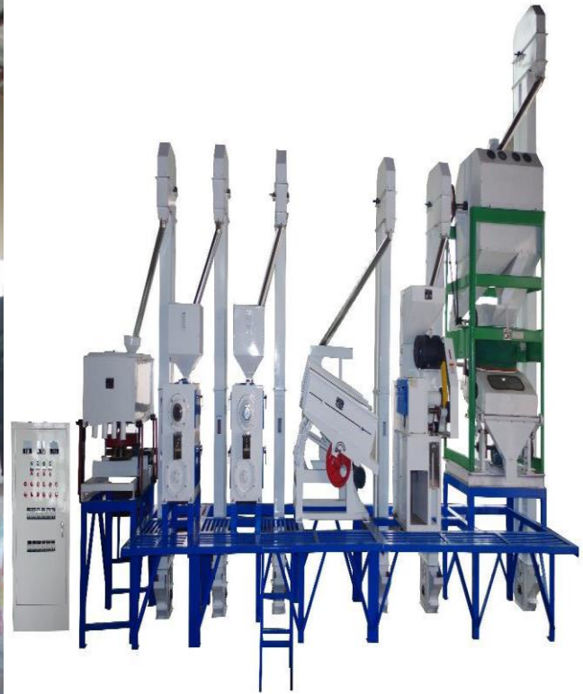
Multi stage rice milling - using semi integrated modular rice mills
