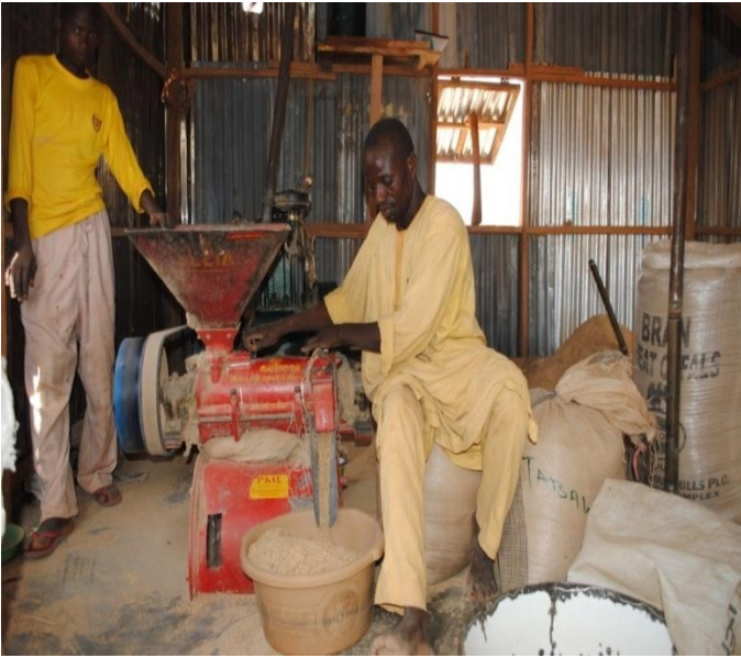
Single pass Rice milling and polishing -using engleberg and improved machines
