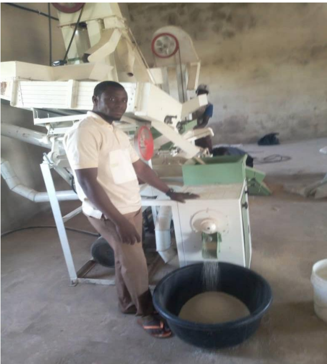
Two Stage/pass rice milling with modular/compact rice mills
